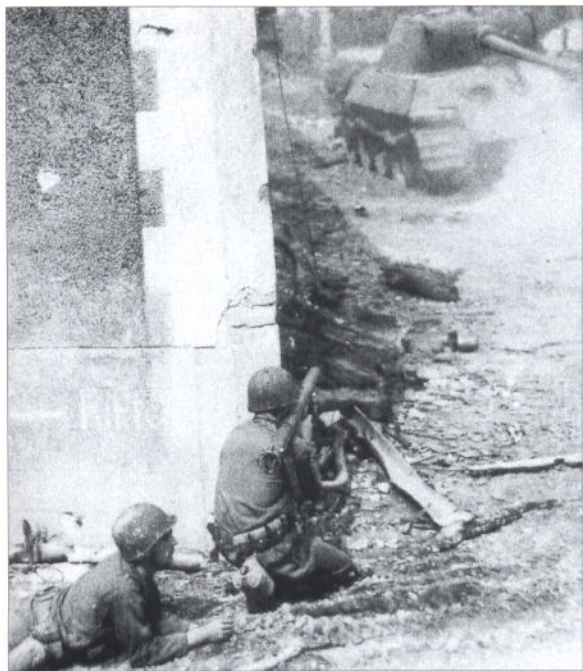
The ultimate mobility for an infantry AT weapon was to be portable by an infantryman over any terrain. In this staged shot a US bazooka crew 'engage' a Panther PzKw V Ausf A with the 2.36in M1A1 rocket launcher, whose light weight and handy size made it easy to manoeuvre into a favourable firing position – unlike that chosen by this photographer for his reconstructed drama: facing the Panther's massive, sloped frontal armour, and inviting fire from its co-axial and bow machine guns.
